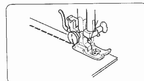
The stitch is sewn with two stitches forward and one stitch backward forming a seam that does not rip easily.
