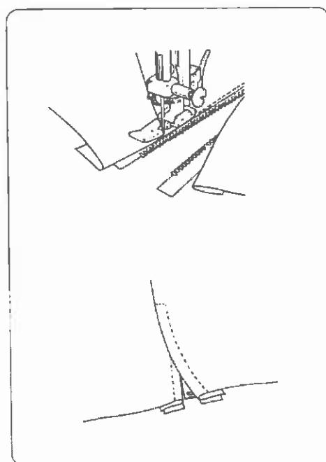
Pin or baste zipper tape to fabric and place it under the foot.
