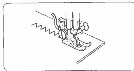
Simple zigzag stitching is widely used for overcasting, sewing on buttons, etc.
