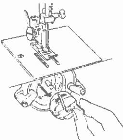
When inserting the bobbin case, place the horn into the recess of the hook race.
