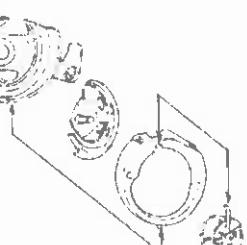
Open the hook race ring holders and remove the hook race ring.
