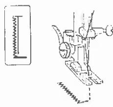
Set the pattern selector dial at " 3 ", sew 5 stitches of bartack and raise the needle from the fabric.
