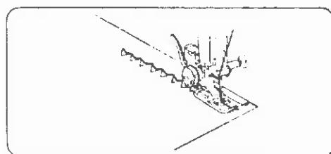
If forward and reverse feeds become unbalanced due to the type of fabric, restore the balance by turning the stitch length dial as follows:
