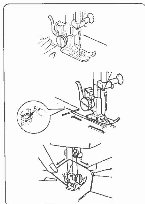
Raise the presser foot and position the fabric next to a stitching guide line on the needle plate.
