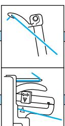
Loosen right needle thread (red)
