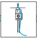
Tighten right needle thread. (red)
