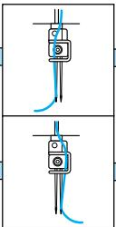
Loosen left needle thread. (orange)
