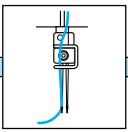
Tighten left needle thread. (orange)
