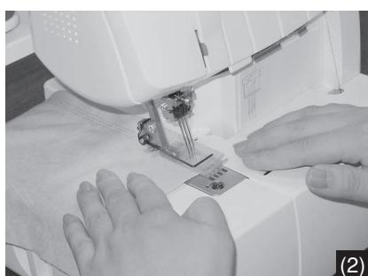
(2) Lower the presser foot, turn the handwheel toward you a few times by hand, and then lightly step on the foot controller to start sewing.
