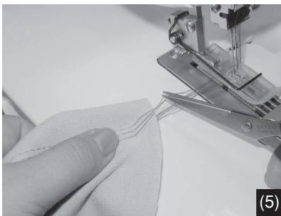
(5) Cut the needle thread which comes out on the upside of the fabric.
