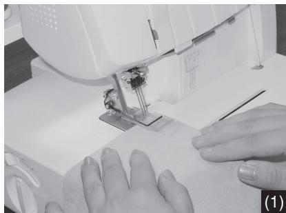
(1) Raise the presser foot, and then place the fabric at the needle drop position.
